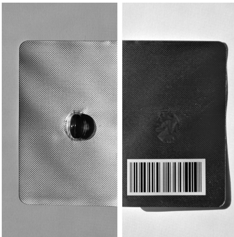
Fig. 1. Blister pack containing PEG marker capsule and barcode identifying its unique constituents.
